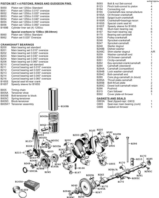
Leaks from crankshaft. One of the most common complaints concerning these engines is loss of oil from the rear of the crankshaft, which incorporates a return scroll designed to feed surplus oil back into the sump via a drain tube in the rear main bearing cap. This antiquated system worked reasonably well when the cars were new provided one accepted a few drops of oil from the split pinned drain hole under the rear of the sump.
